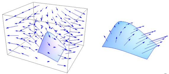
For each infinitesimal piece of the surface, we have an infinitesimal area vector dA as shown in the figure below on the left. For each infinitesimal piece of the surface, the corresponding infinitesimal area vector points perpendicular to the surface (at that piece) and its magnitude gives the area of that piece. A sampling of these along the surface is shown in the figure on the lower right along with the vector field along the surface.
