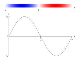
Figure 4: Charge distribution for Example 2.
